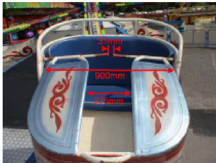
Photograph 4 Front view of the Octopus ride, showing the widths of the passenger car and width of the gaps in the containment.
