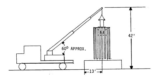
6. Raise cylinder out of the top of the ride, observing clearance of plumbing, through mounting hole, as it is removed. Lower cylinder to a pallet on the ground, protecting the plumbing and bar linkage as it is being placed onto the pallet.
