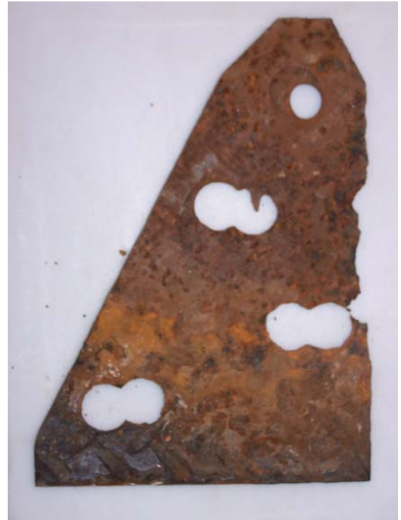
This part shows the beginning of the deterioration process. This part is also unacceptable.
