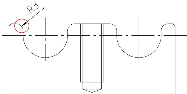
Smoothening of the edges can be done using either sand paper or grinding tools. Keep in mind to only use soft abrasives on power tools in order not to harm the pulley's existing groove structure.
