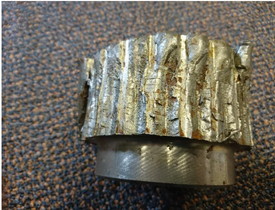
▲ Failed original pinions
