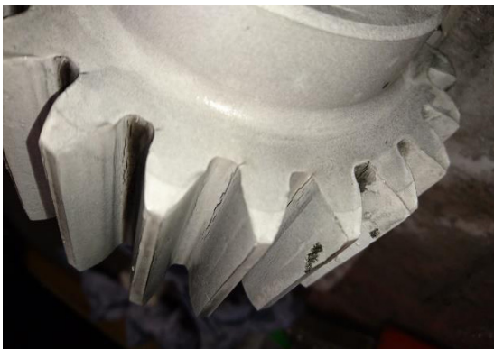
▲ Failed replacement pinions
