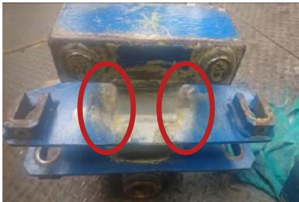
▲ Reverchon Spinning Coaster cracking
