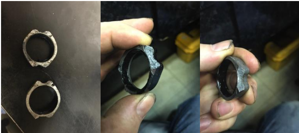
The above images show the two failed seal retaining caps. Both have had their bolting lugs sheared completely off.
